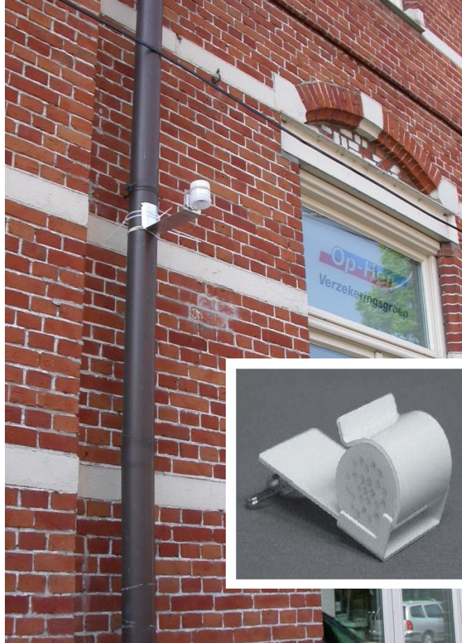
Measurement of nitrogen oxides with passive samplers
