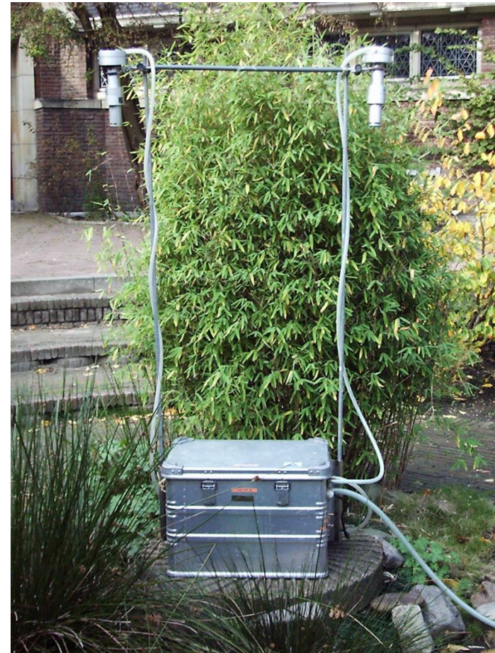
Measurement of fine particles with pump and sampling head
