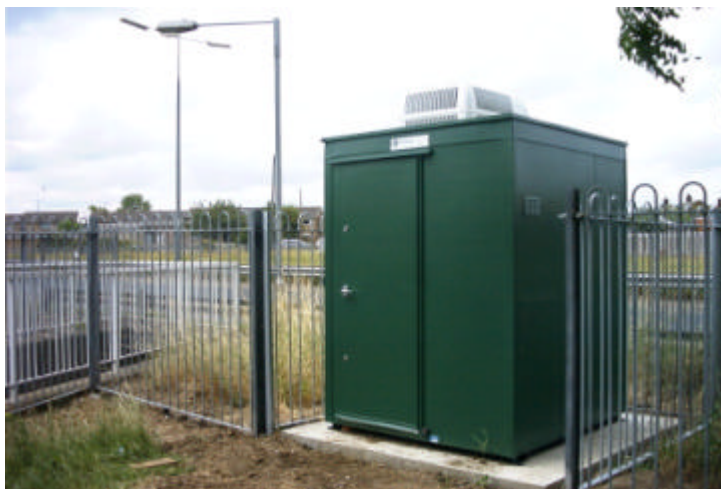
Figure 22 The Thurrock 3 roadside site joined the LAQN during August and measures \text{NO}_x , \text{SO}_2 and \text{PM}_{10} (TEOM).
