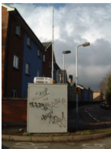
Figure 13 The Hillingdon 2 site that became fully operational during April. The site monitors \text{NO}_x and \text{PM}_{10} (TEOM) at a roadside location close to Hillingdon Hospital.
