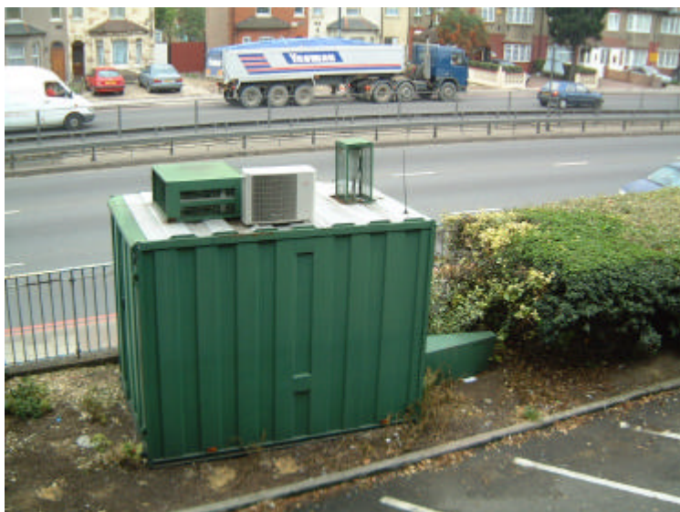
Figure 12 The Brent 4 site that joined the LAQN during June as a replacement for Brent 2. The site is located on the A406 around 300 m from the location of Brent 2. The site monitors \text{NO}_x , \text{SO}_2 and \text{PM}_{10} (TEOM).
