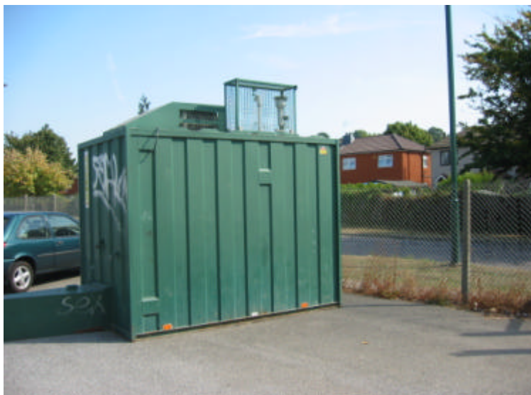
Figure 14 The Waltham Forest 3 site that joined the network during July. The site is located in a roadside location in Chingford and measures \text{NO}_x , \text{SO}_2 and \text{PM}_{10} (TEOM).
