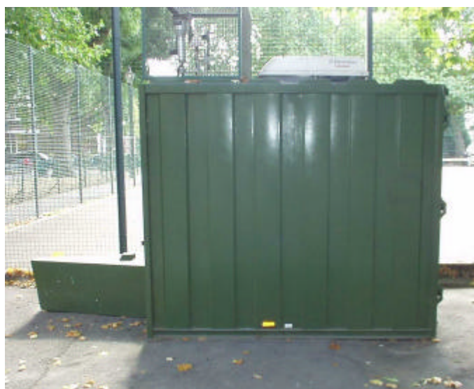
Figure 17 The Hammersmith & Fulham 2 background site that joined the LAQN during July. The site monitors \text{NO}_x and \text{PM}_{10} (TEOM).
