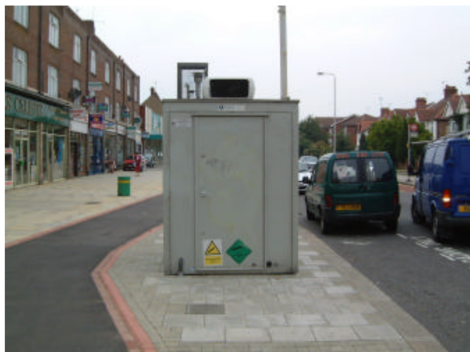
Figure 16 The Harrow 2 site that joined the LAQN during June. The site is located in a roadside location and monitors \text{NO}_x and \text{PM}_{10} (TEOM).
