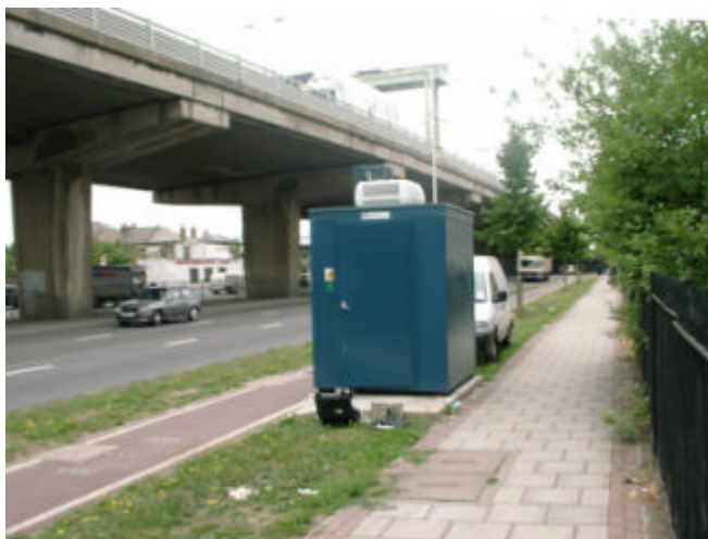
Figure 18 The Hounslow 5 roadside site that replaced Hounslow 1 during August. The site is located beside the A4 and M4 and monitors CO, NO x and PM 10 (TEOM).
