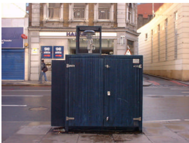
Figure 19 The Lambeth 4 roadside site that joined the LAQN in December. The site measures NO x , SO 2 and PM 10 (BAM) alongside the A23 in Brixton.
