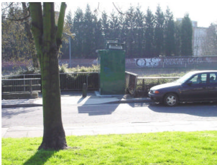
Figure 23 The Redbridge 5 site also joined the LAQN during 2003. The site was installed in November as a replacement for Redbridge 2 that closed during April. The site measures \text{CO} , \text{NO}_x and \text{PM}_{10} (BAM).
