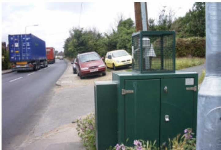
Figure 20 The Reigate and Banstead 2 NO x site that joined the LAQN during August. The site is located in a suburban area immediately adjacent to Gatwick Airport. The site forms part of a larger monitoring programme, which also includes Reigate and Banstead 1, and aims to quantify NO 2 around the airport.
